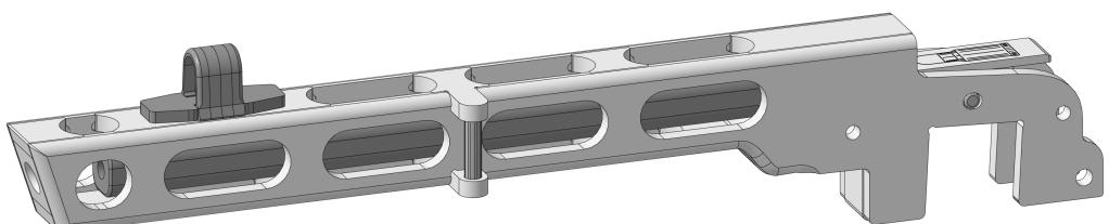
**!** Insert the pin into the hole to adjust the parts before gluing. **Make sure the glue doesn't get on the pin.** After drying of the glue, the pin should be easily removed. Carefully file down the sides.
